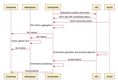
Figure 34 UC5 Sequence Diagram
