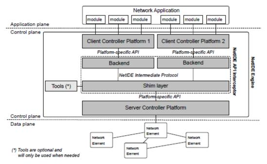
Figure 18. NetIDE Network Engine Architecture
