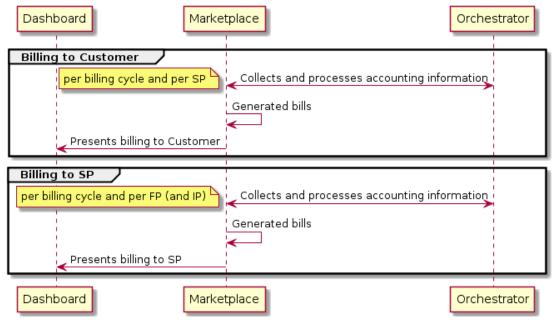
Figure 36. UC5 Sequence Diagram
