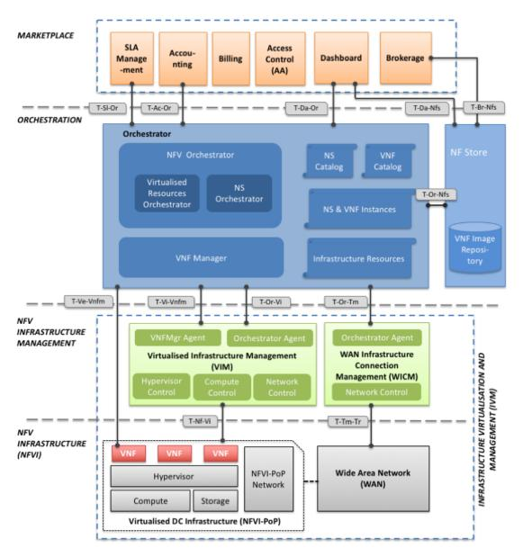
Figure 20. High-level view of overall T-NOVA System Architecture
