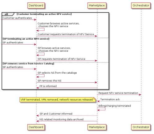
Figure 37 UC7 Sequence Diagram
