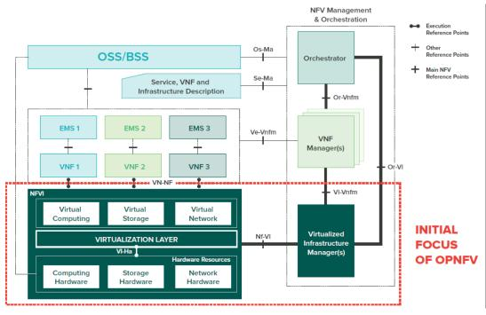
Figure 3. OPNFV mapping to ETSI reference architecture
