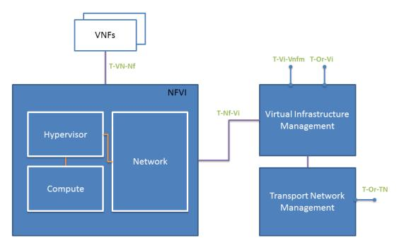
Figure 24. High-level architecture of T-NOVA IVM.
