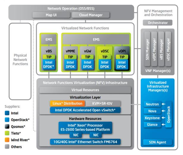
Figure 7. Intel NFV High Level Architecture
