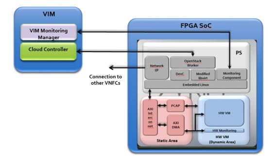
Figure 8. Monitoring architecture for the T-NOVA FPGA SoC
