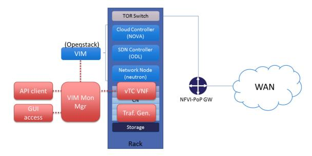
Figure 12. Testbed configuration for testing VIM Monitoring
