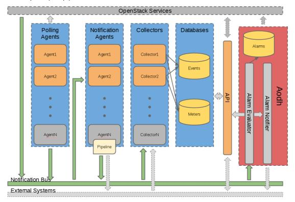
Figure 1. OpenStack Telemetry/Ceilometer architecture
