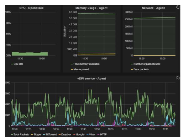
Figure 13. End-to-end functional test: the VIM MM GUI screenshot, integrating metrics from various sources
