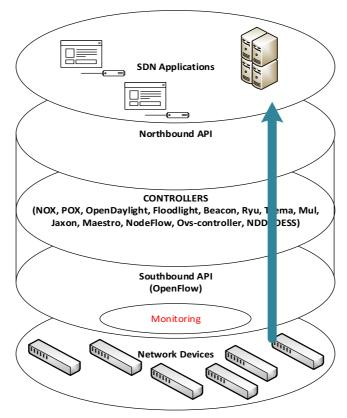
Figure 16. Communication of monitoring metrics in an OpenFlow-enabled architecture
