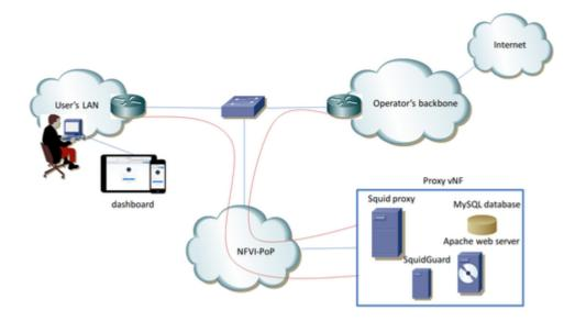
Figure 30. PXaaS high level architecture
