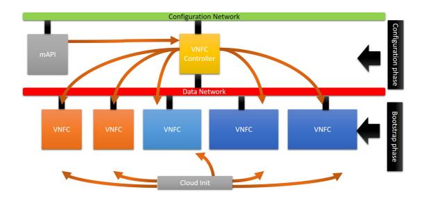
Figure 8. Two-phase VNF configuration
