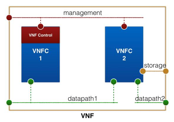
Figure 6. Virtual Link VNFC interconnection example.
