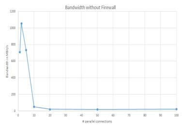
Figure 12. Throughput without firewall
