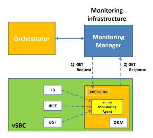
Figure 9. Monitoring data handling (via snmp) in case of vSBC
