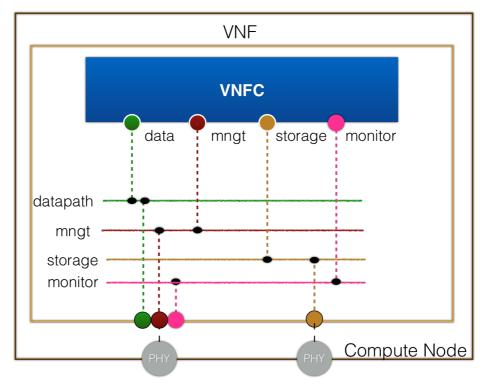
Figure 3 VNF/VNFC Virtual Links and Connection Points
