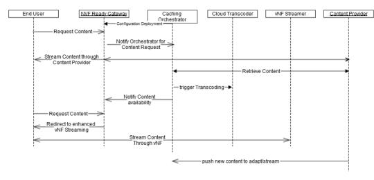
Figure 26 Sequence diagram for the transcode/stream VNF example.
