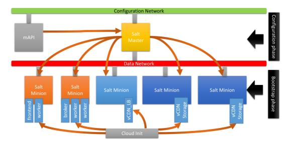
Figure 28 vCDN implementation for Software configuration Management.
