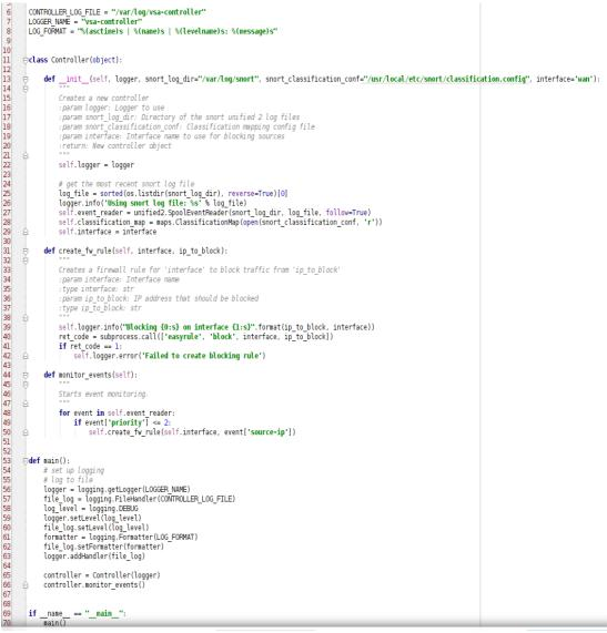
Figure 11. A sample of code of the FW Controller
