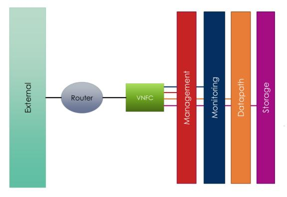
Figure 4. OpenStack overview of the T-NOVA VNF deployment networks.
