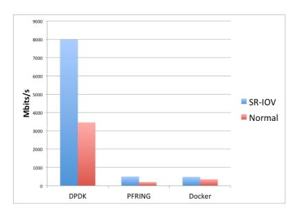
Figure 22. vTC Performance comparison between DPDK, PF\_RING and Docker
