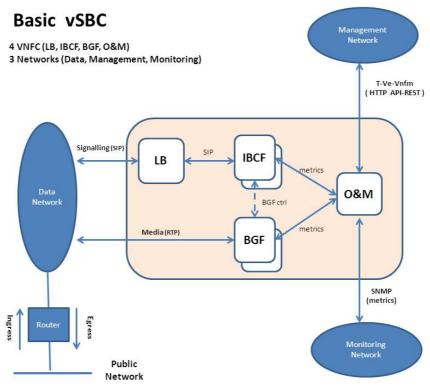
Figure 16. Basic vSBC internal architecture.
