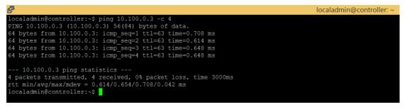
Figure 12 Inter-PoP connectivity test
