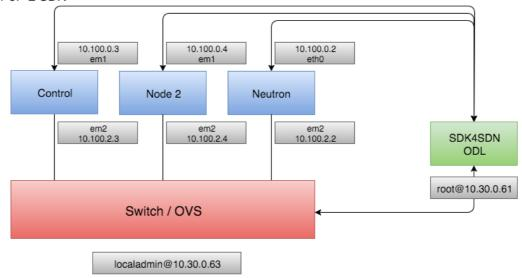
Figure 18 OpenStack and OpenDaylight nodes in Athens testbed
